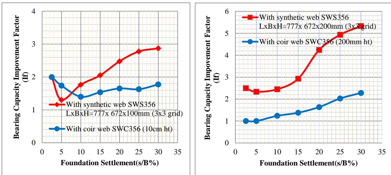
Figure 5. BCIF Vs Foundation settlement for web SW356 (a) for 100 mm height and (b) for 200 mm height
