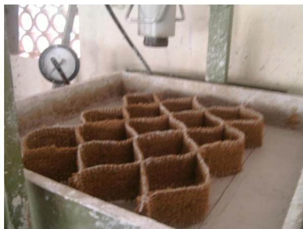
Figure 2. Coir geocell above soft clay bed
