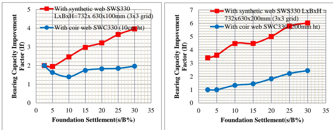
Figure 3. BCIF Vs Foundation settlement for web SW330 (a) for 100 mm height and (b) for 200 mm height
