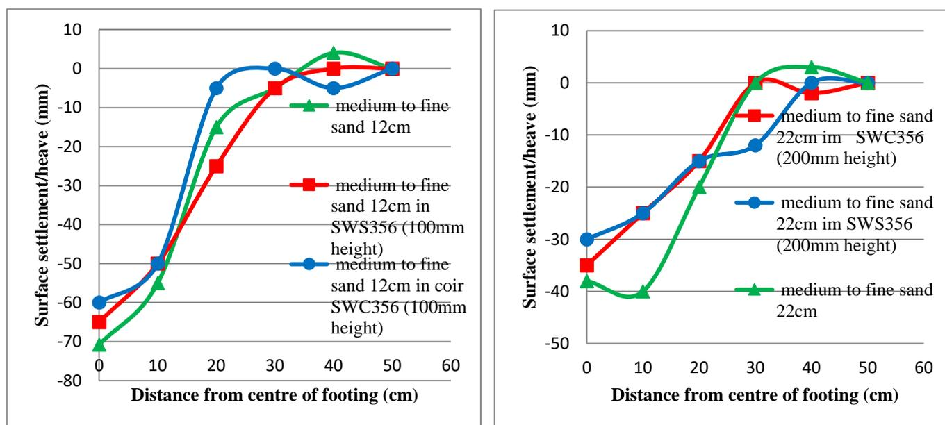
Figure 6. Settlement or heave from the centre of footing for SW356 (a) for 100 mm and (b) for 200 mm height
