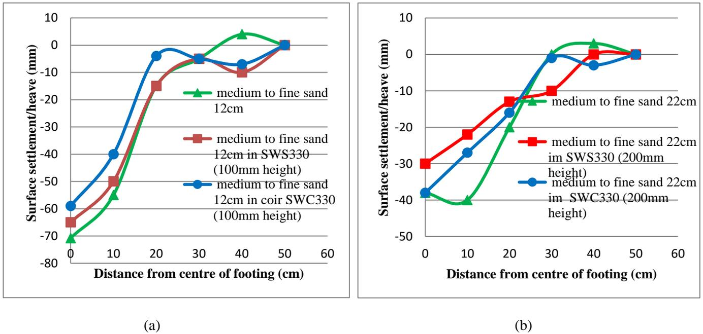
Figure 4. Settlement or heave from the centre of footing for SW330 (a) for 100 mm and (b) for 200 mm height
