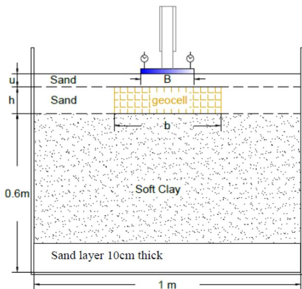
Figure 1. Schematic diagram of test set up
