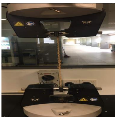
Figure 3. Tensile strength of netting fiber
