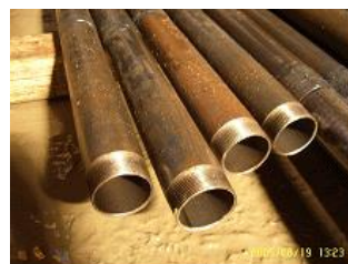
(b) Hollow steel pipe for GPM
