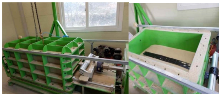
Figure 3 Pullout Test Equipment
