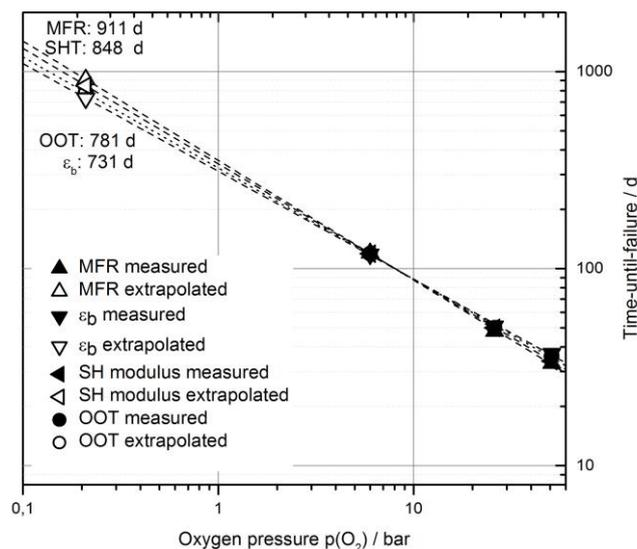
Figure 10. Time-until-failure as function of oxygen pressure.
