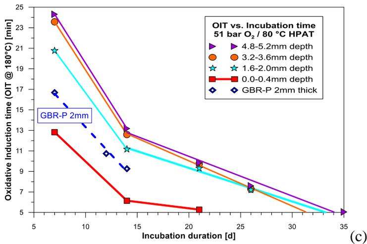
Figure 2. OIT (at 6 bar (a), 26 bar (b), 51 bar (c) oxygen pressure) in different depth of a 10 mm thick plate in comparison with a 2 mm thick GBR-P.
