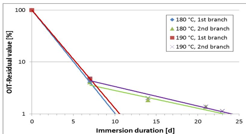
Figure 4. OIT-Residual value of PE-HD GBR-P at 26 bar and 80 °C
