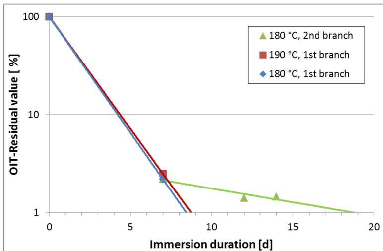
Figure 5. OIT-Residual value of PE-HD GBR-P at 51 bar and 80 °C
