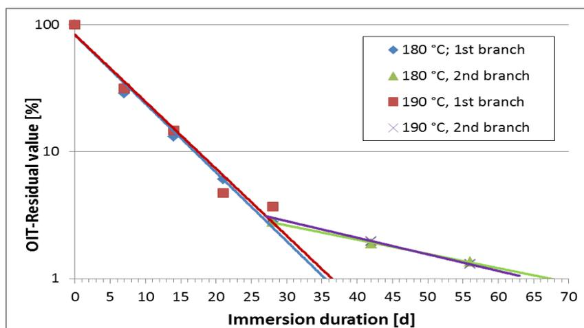
Figure 3. OIT-Residual value of PE-HD GBR-P at 6 bar and 80 °C
