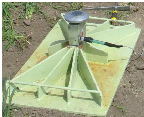
Figure 1. Mechanical adapter and load cell for introducing impulse force into the soil
