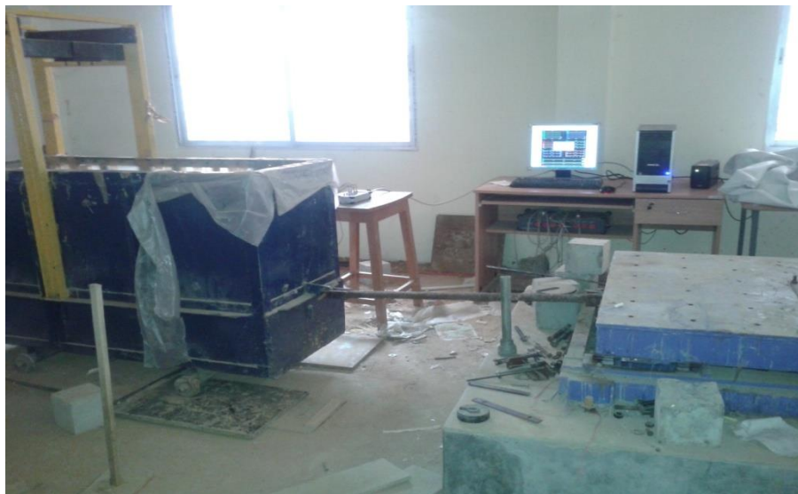
Figure 4. Shake table set up with laminar box
