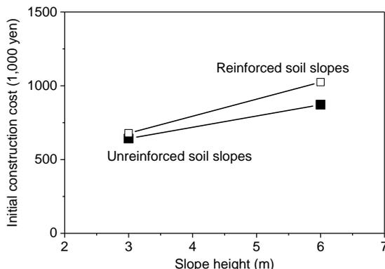
Figure 2. Initial construction cost of unreinforced and reinforced soil slopes
