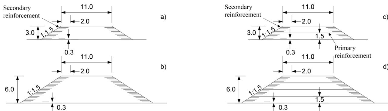
Figure 1. Analytical models of unreinforced and reinforced soil slopes: a) unreinforced soil slope with height of 3.0 m, b) unreinforced soil slope with height of 6.0 m, c) reinforced soil slope with height of 3.0 m, d) reinforced soil slope with height of 6.0 m.
