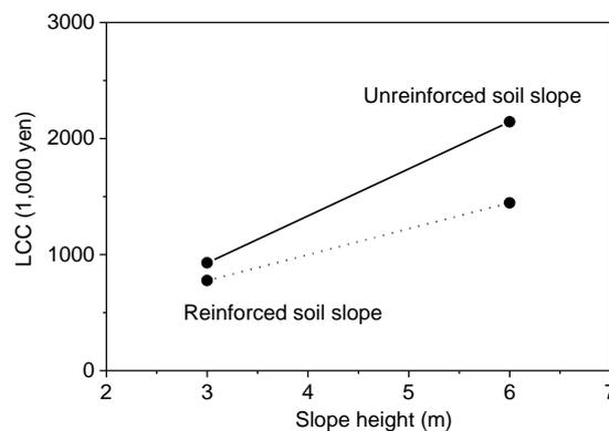
Figure 6. LCC of the unreinforced and reinforced soil slopes with 75% confidence value of seismic residual displacement
