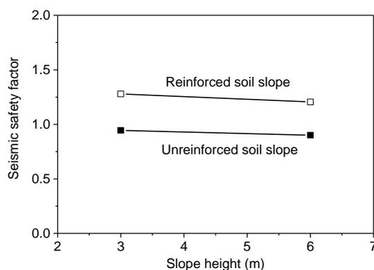
Figure 4. Seismic safety factor of unreinforced and reinforced soil slopes
