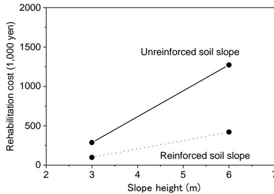
Figure 5. Rehabilitation cost of the unreinforced and reinforced soil slopes with 75% confidence value of seismic residual displacement
