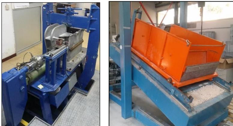
Figure 5. Picture of the large scale shear box device (left) and the large scale inclined plane device (right) in Irstea Aix-en-Provence.
