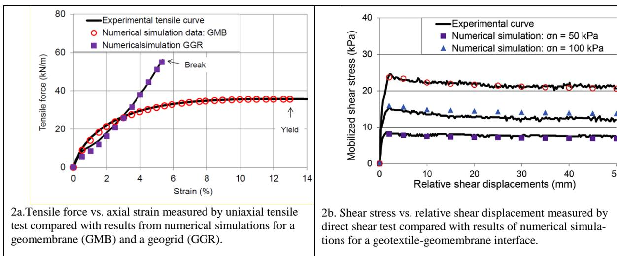
Figure 2. Comparison between experimental curves and numerical simulation (Tano et al. 2017).
