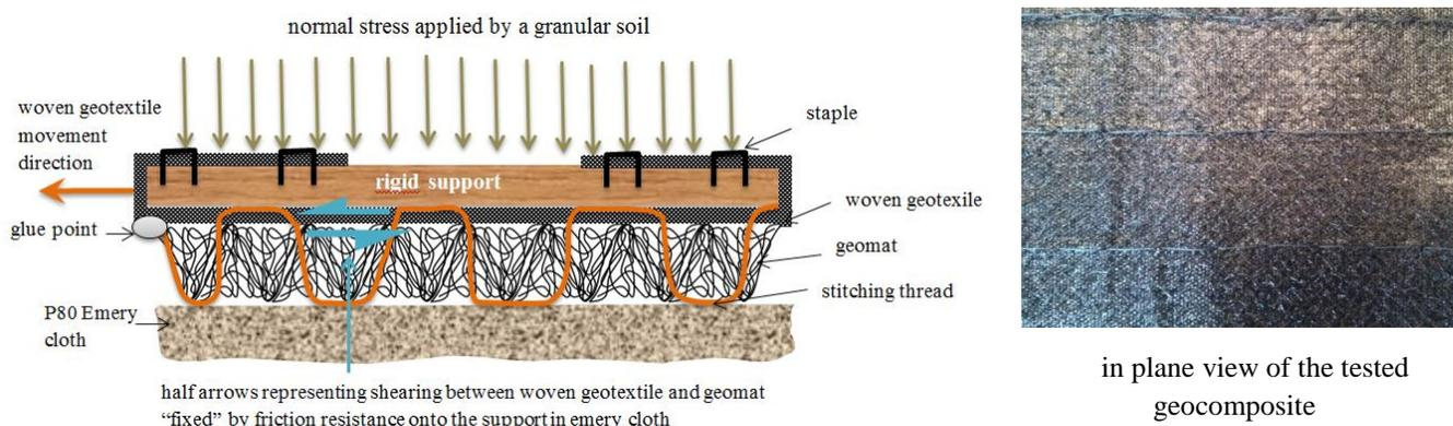
Figure 7. Schematic representation of the testing method to assess the internal shear resistance of a geocomposite with an in-plane view in the picture on the left (Stoltz and Hérault, 2016).
