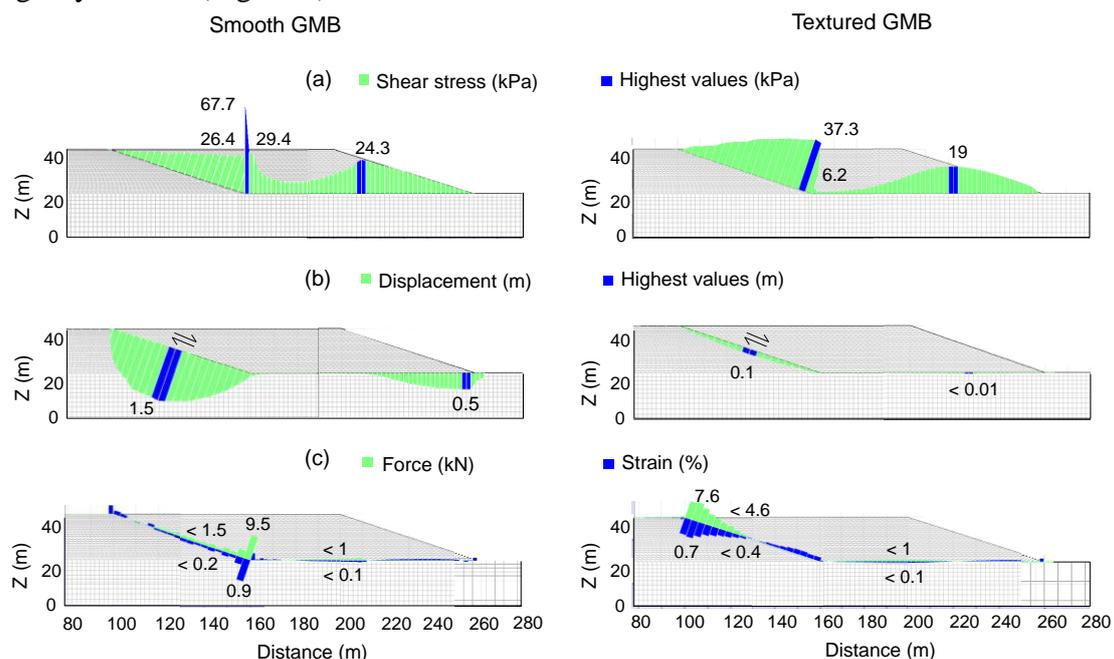
Figure 4. Comparisons between smooth GMB and textured GMB at H=20 m. (a) Shear stress along critical interface, (b) displacements along interface I2, (c) force and strains in geomembrane (Tano et al., 2017b).
