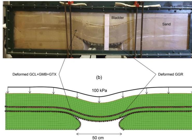
Figure 3. Overall deformed shape of reinforced lining system: (a) experiment, (b) numerical model (Tano et al., 2017a).
