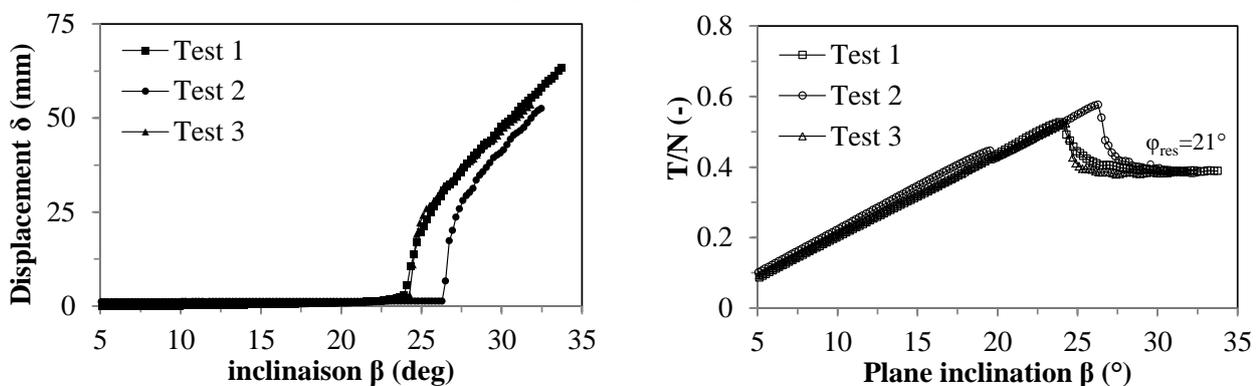
Figure 6. Example of results from the residual friction testing procedure using an IP device (Stoltz et al. 2012).
