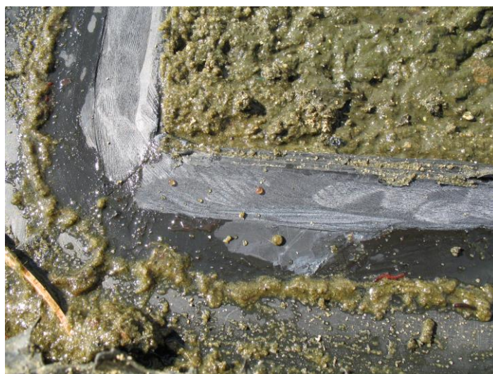
Figure 15. Grinding gouges on unmelted surface.
