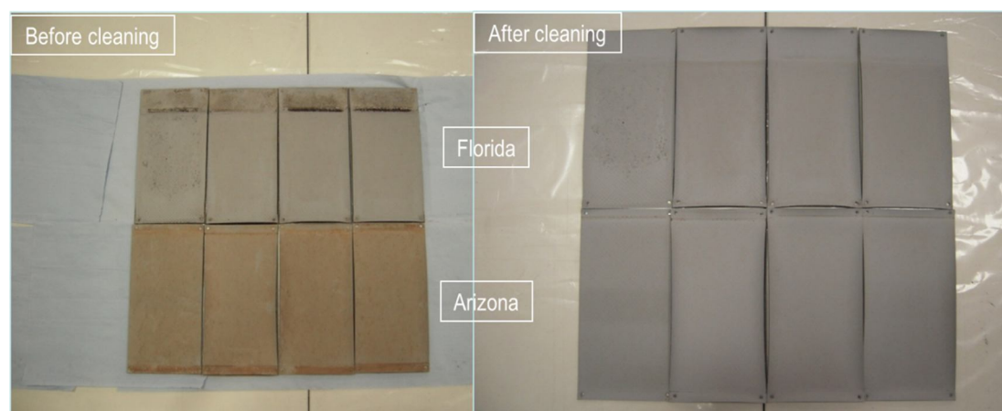
Figure 2. Florida and Arizona samples after 10 years of exposure, before and after cleaning.
