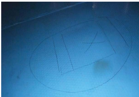
Fig. 14 Separation of liner from base as a result of air bubble at domed centre.
