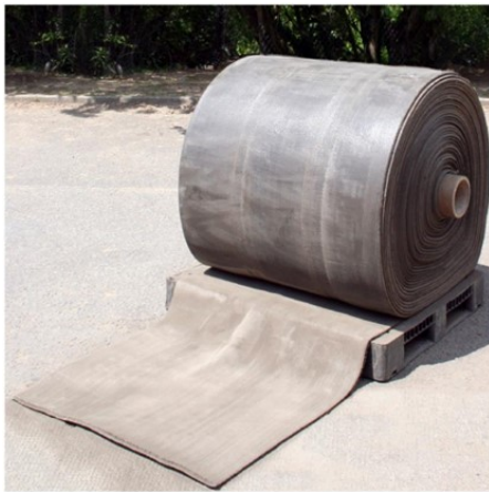
Figures 4 and 5. Typical packaging of GCCMs, makes them easier and cheaper to transport than conventional concrete.
