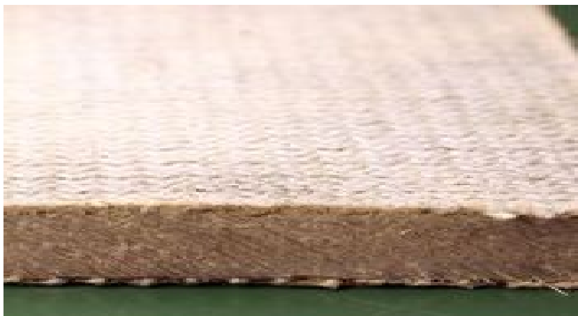
Figure 1. Cross section of 8mm GCCM showing various component
