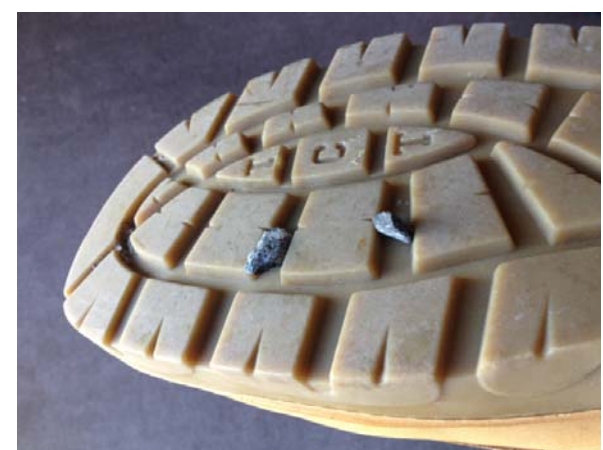
Figure 22. Stones in tread of work boots causing puncture of geomembranes [Scheirs]
