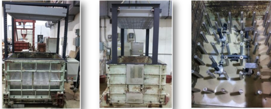
Figure 1: Test set up for laboratory model test (front view, side view, plan view from the left to right)
