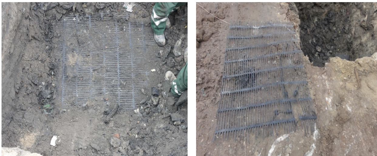
Fig. 4. Geogrid HDPE samples collected after 20 years of service
