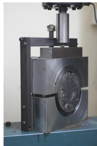
Figure 3. Leutner Shear test setup
