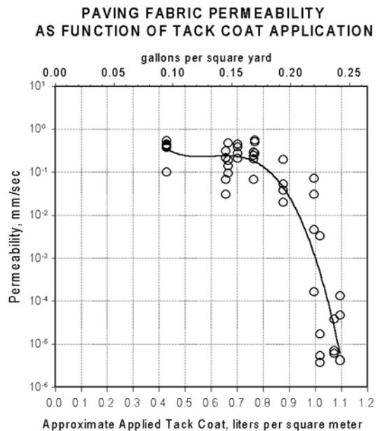
Fig 2 Barrier-function of tack coat (Suits et al. 1999)
