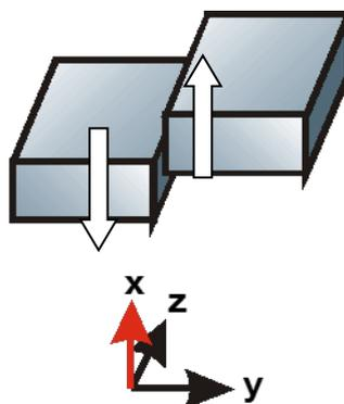
Fig 12 vertical shear stress
