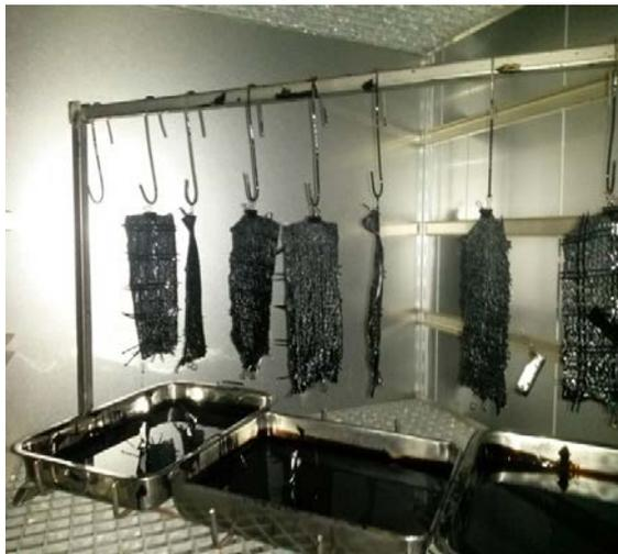
Fig. 1 Bitumen retention test
