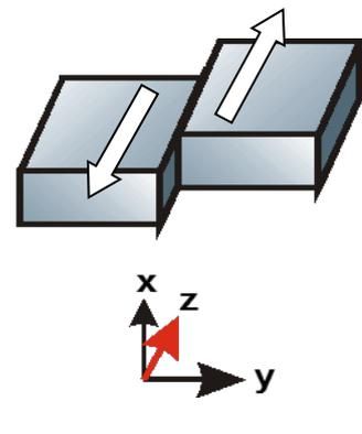
Fig 13 In-plane shear
