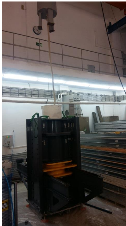
Figure 5. Pluviation of sand into the testing assembly
