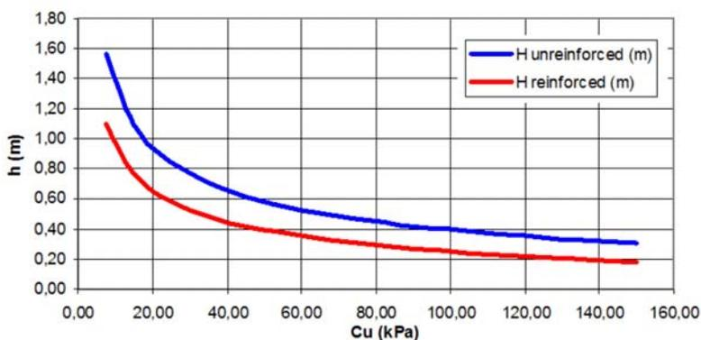
Figure 2. Typical plot of the required platform thickness (H) versus the undrained cohesion  $c_u$  of the subgrade considering a reinforced (red line) and unreinforced (blue line) platform.
