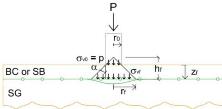
Figure 4. Scheme of the first geogrid layer
