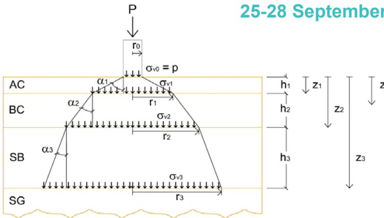
Figure 3. General scheme of the multi-layers model with different soil characteristics
