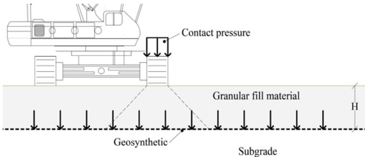
Figure 1. Static Method considers uniform load on a rectangular loaded area
