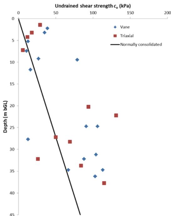
Figure 5. Derived values of undrained shear strength from the available ground investigations
