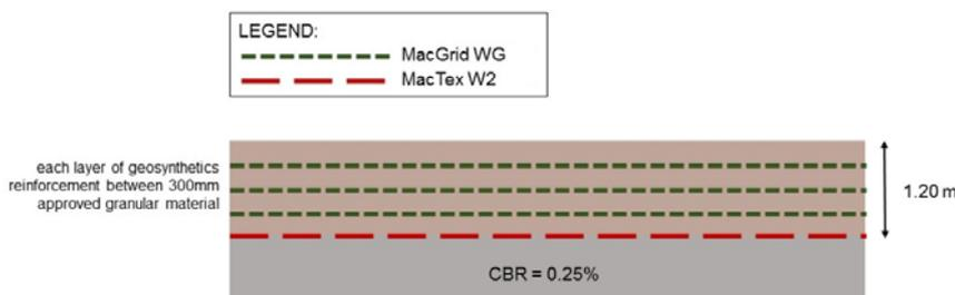
Figure 6. Working piling platform supporting the piling machine with a design thickness of 1.20m
