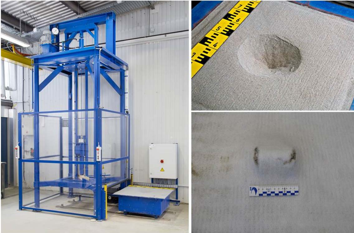
Figure 3: Drop test facility (left), deformation in the sand bed (top right) and a punctured sand mat (below right)
