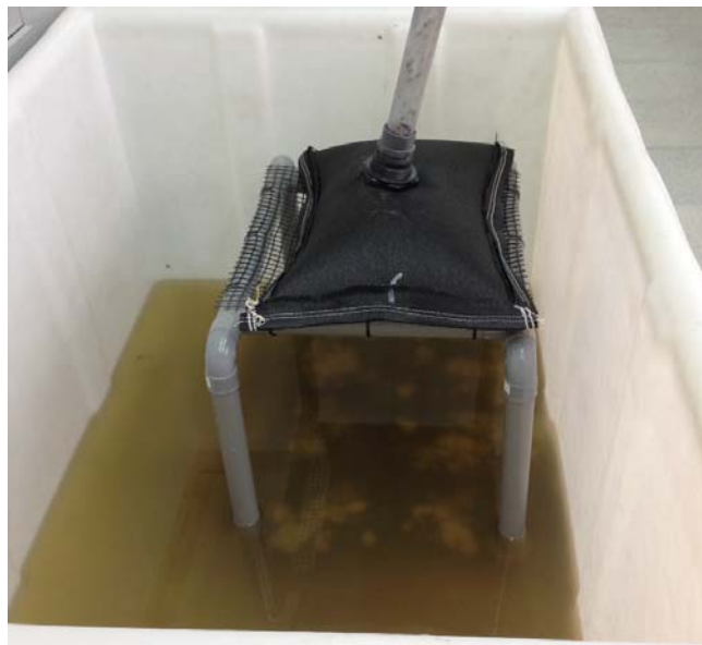
Figure 1. Geotube Dewatering System (The GDT system)
