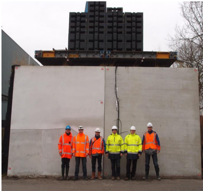
Figure 3: Test load of 250 kPa at the test site KWS cube, Utrecht, using calibrated weights
