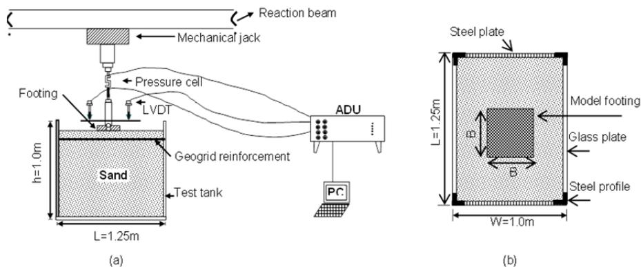
**Figure 2.** Test tank and apparatus used in the experimental study
