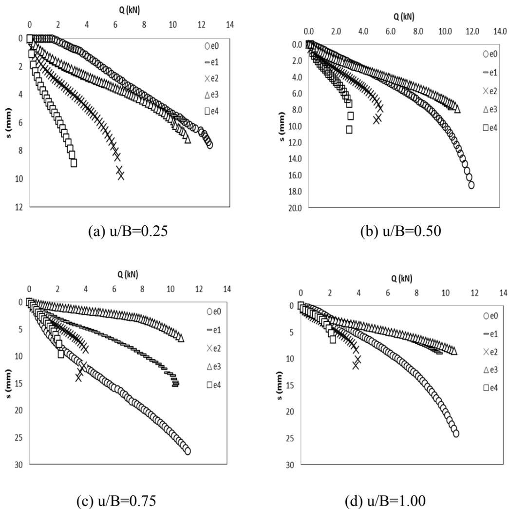
**Figure 4.** Vertical load - settlement curves for different  $u$  values
