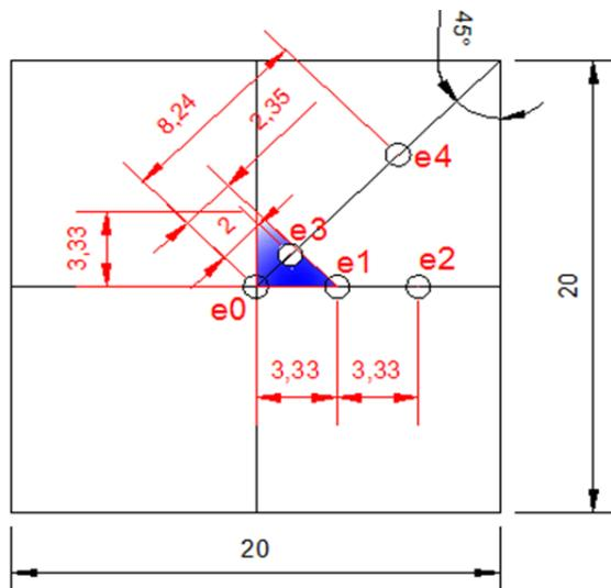
**Figure 1.** Model square footing and loading points (dimensions in cm)
