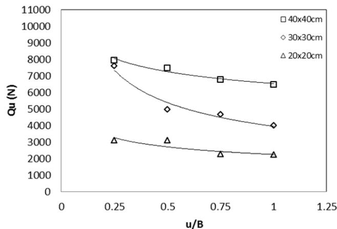
**Figure 6.**  $u/B - Q_u$  curves for different footing widths with constant eccentricity ( $e_4$ )
