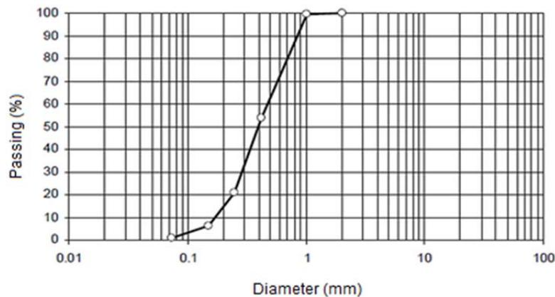
**Figure 3.** Grain size distribution curve of the sand
