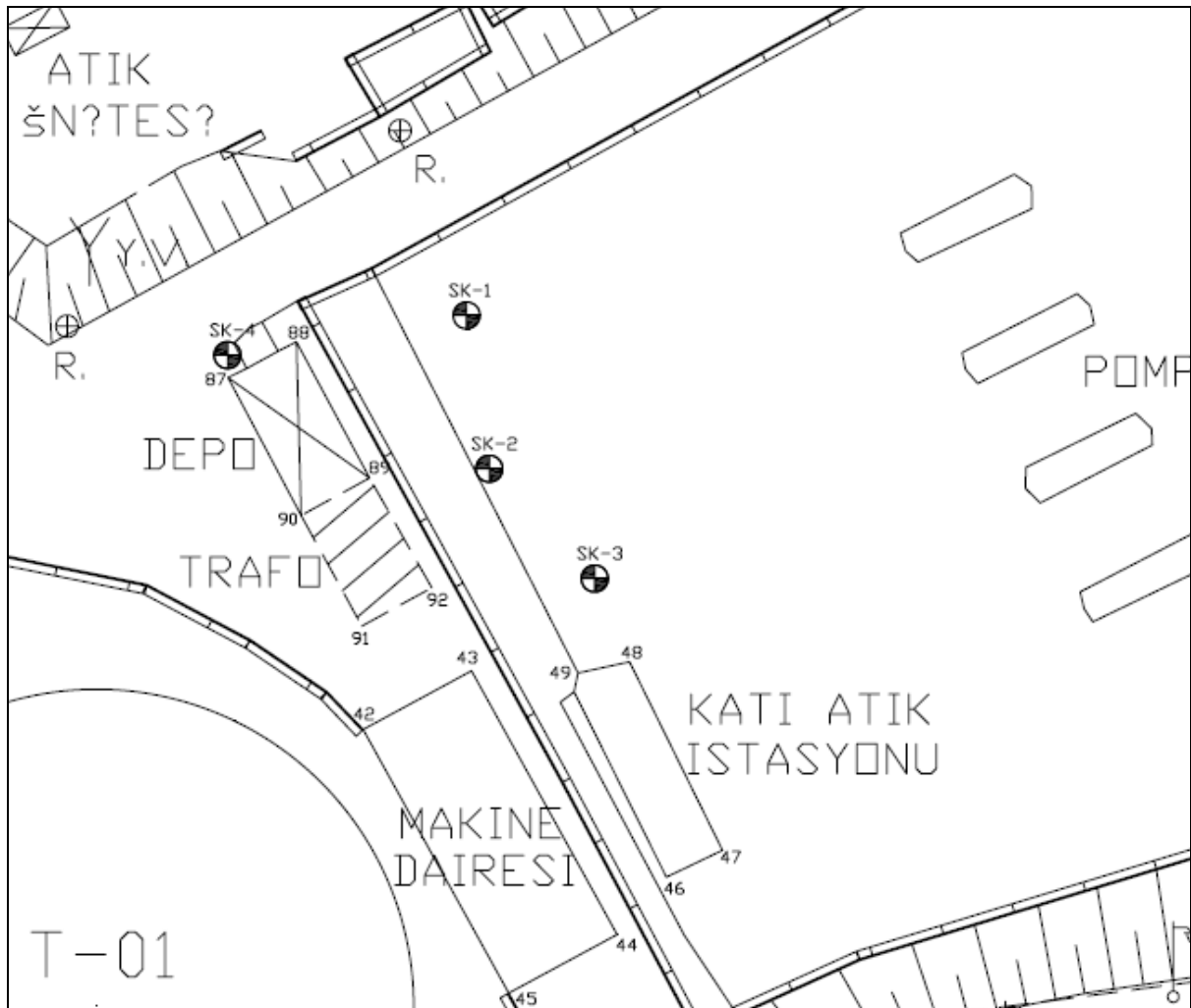
Figure 4: Layout of the soil investigation boreholes
