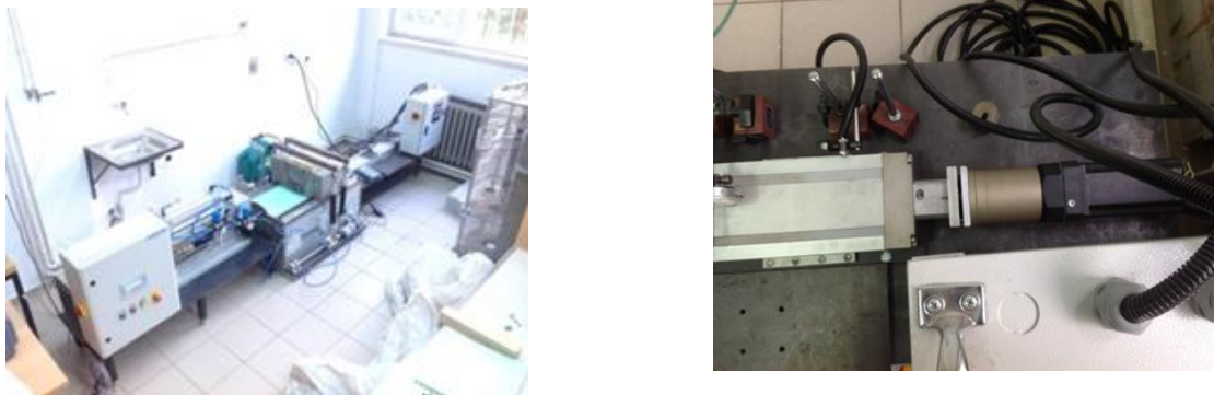
Figure 6: General view of the large displacement direct interface test device and the linear actuator driven by the step motor and reduction gear mechanism (right)
