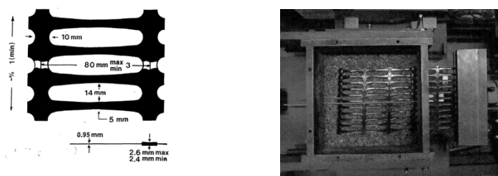
Figure 3: The geogrid used and its placement into the box
