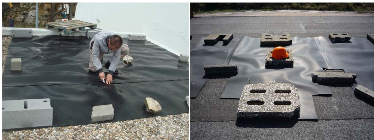
Figure 1: Examples of geomembrane samples exposed to climatic conditions
