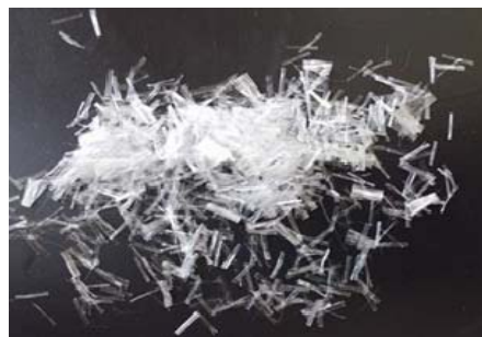
Figure 2: 6 mm long fibers used in this study
