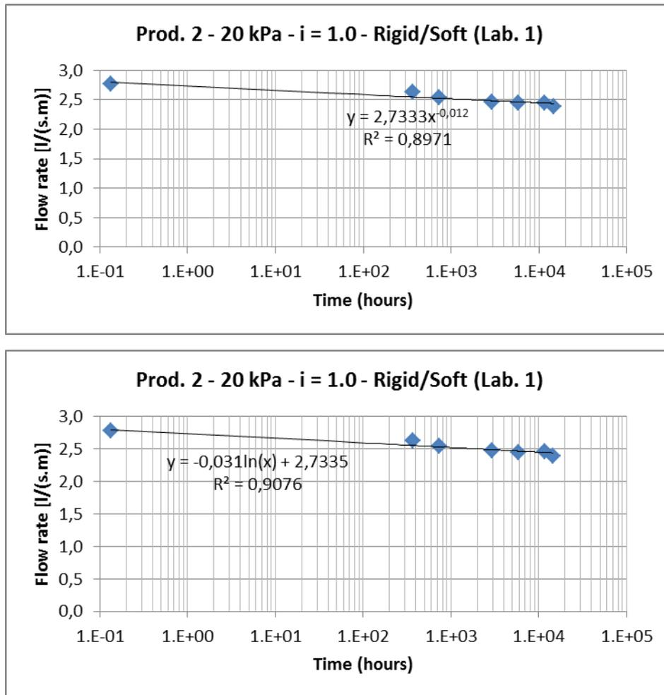
Figure 3. Similar regression curve for logarithmic and power regression in case of semi-compressible monofilament structures
