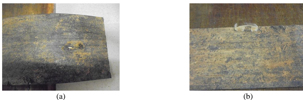
Figure 5: Exhumed samples from the TRL wall showing (a) minor damage (b) some pull through of fibres
