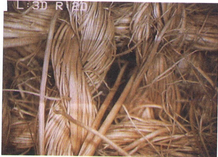
a) Optical microscope view of woven coir geotextile, X28
