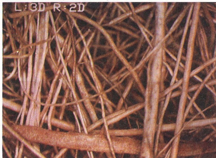
c) Optical microscope view of nonwoven coir geotextile, X28 (with scrim)
