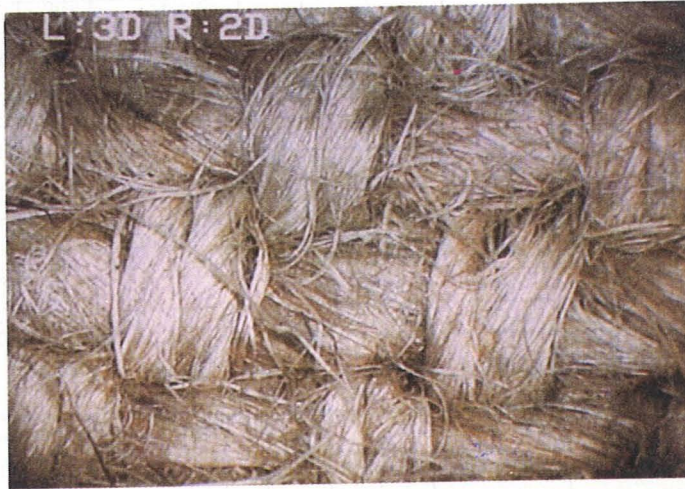
d) Optical microscope view of woven jute geotextile Type A X28
