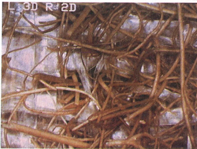
b) Optical microscope view of nonwoven coir geotextile, X28 (without scrim)
