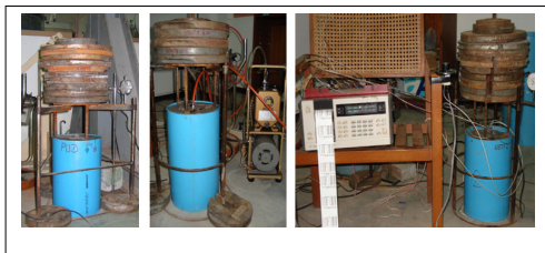
Figure 1. Small scale consolidometer for undisturbed specimens; (a) with PVD, (b) with Vacuum-PVD and (c) with Thermo-PVD
