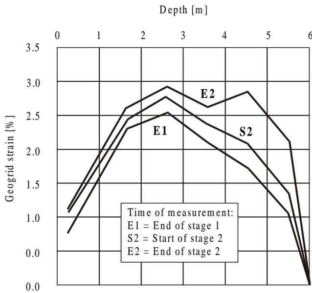
Figure 6. Strains of geogrid (extensometer A)
