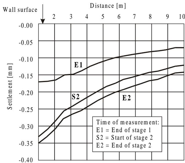
Figure 7. Settlements measured with horizontal inclinometer 2
