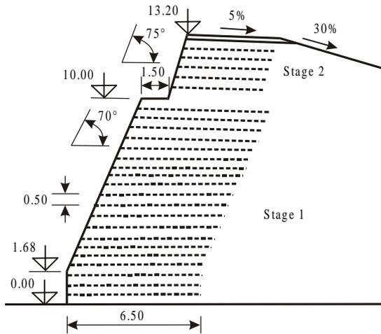
Figure 1. Schematic cross section of the test wall.
