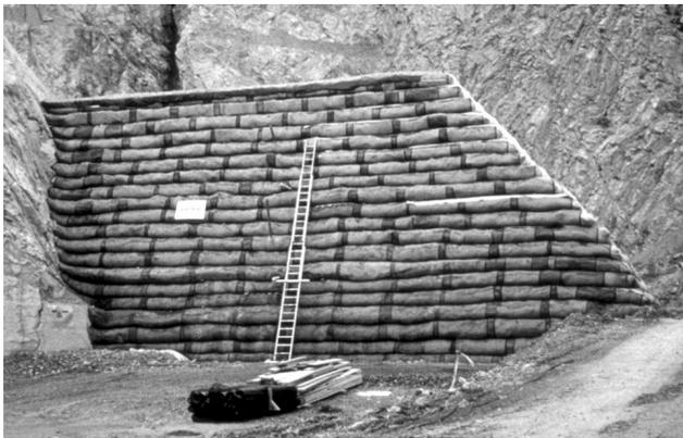
Figure 2. Front view of the instrumented test wall (stage 1).
