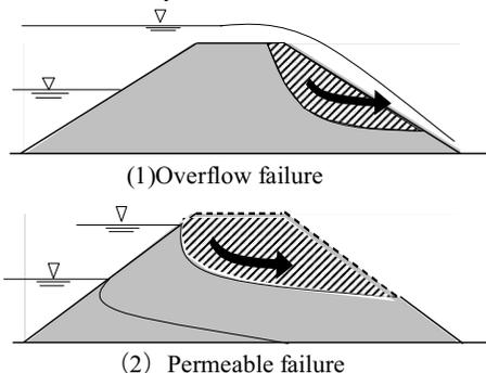
Fig.2. Generally categories, a failure of dyke
