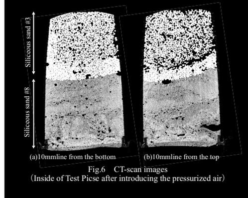
Fig.6 CT-scan images (Inside of Test Piece after introducing the pressurized air)
