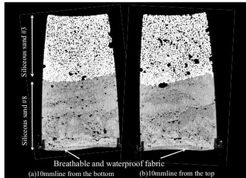
Fig.5 CT-scan images (Inside of Test Piece before introducing the pressurized air)
