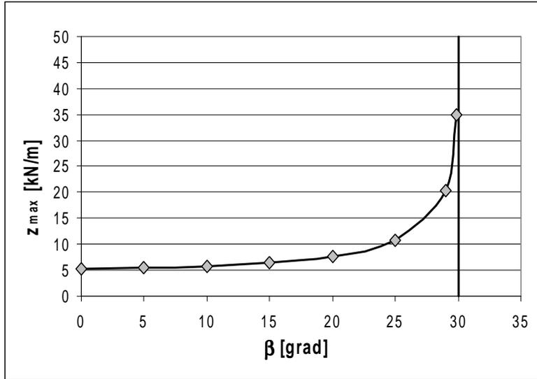
Figure 4. Influence of the inclination of the terrain  $\beta$  for  $\varphi'_s = \varphi'_u = 30^\circ$ ,  $c'_s = c'_u = 0 \text{ kN/m}^2$ ,  $\gamma_s = \gamma_u = 20 \text{ kN/m}^3$
