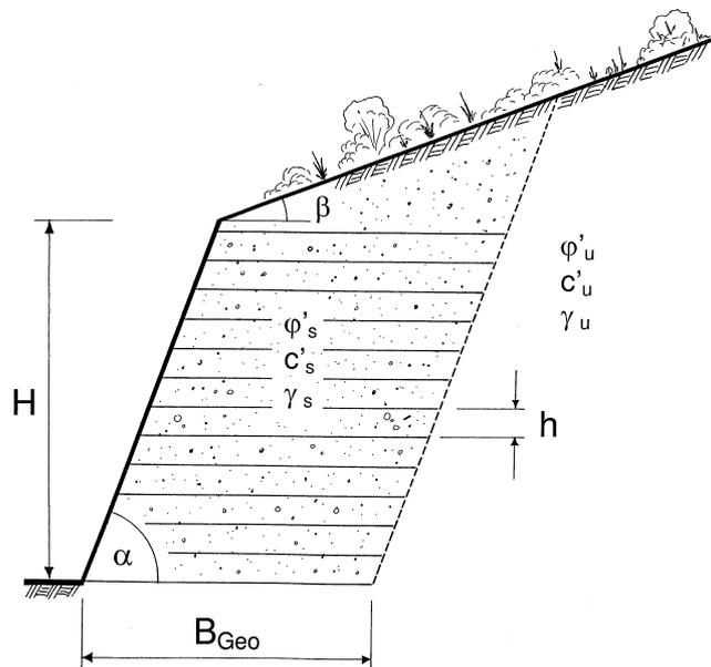
Figure 1. Example of a geotextile-reinforced structure
