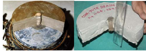
Figure 8. Final consolidated clay sample of 'swd' and 'cjd' of n=11.04 (end of 320kPa pressure)
