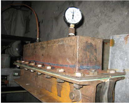
Figure 8. Seepage experiment device of anchoring system.
