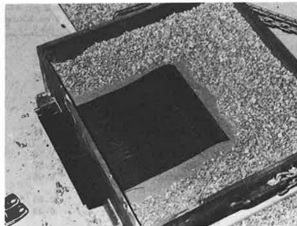
Figure 2: Pullout Test Box with Geomembrane Prior to Testing.
