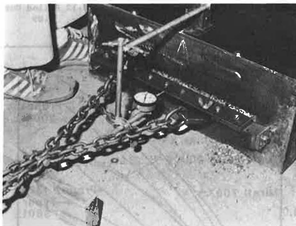
Figure 3: Pullout Test Box with Geomembrane in Grip During Test.
