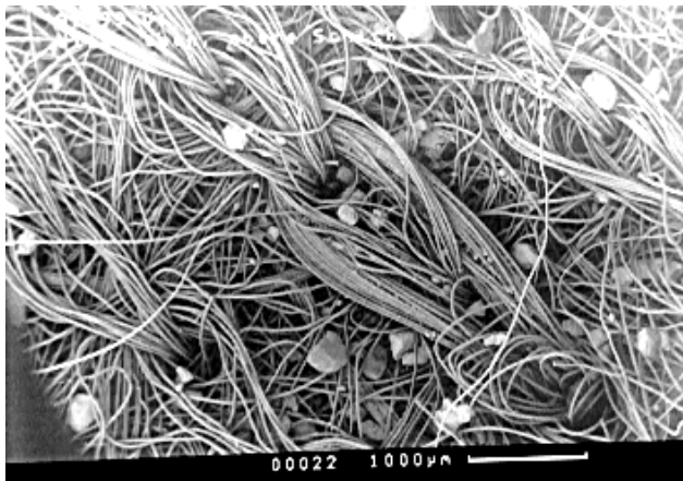
Fig. 9: granular intrusions in the nonwoven filter
