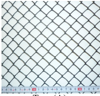
Type(A) Opening: 20×25 mm Nominal tensile load: 1.96×1.96 kN/m Photo 1. geogrids
