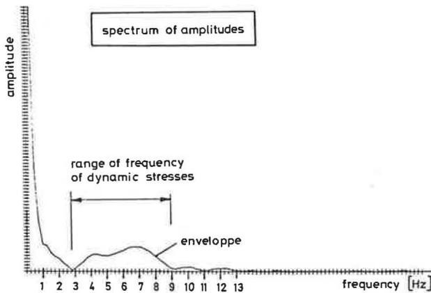
Fig.8: spectrum of amplitudes of stress sequence in Fig.7; determined by Fast Fourier Transformation (FFT)
