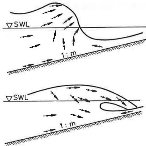
Fig. 1: kinematics of wave run-up on slope
