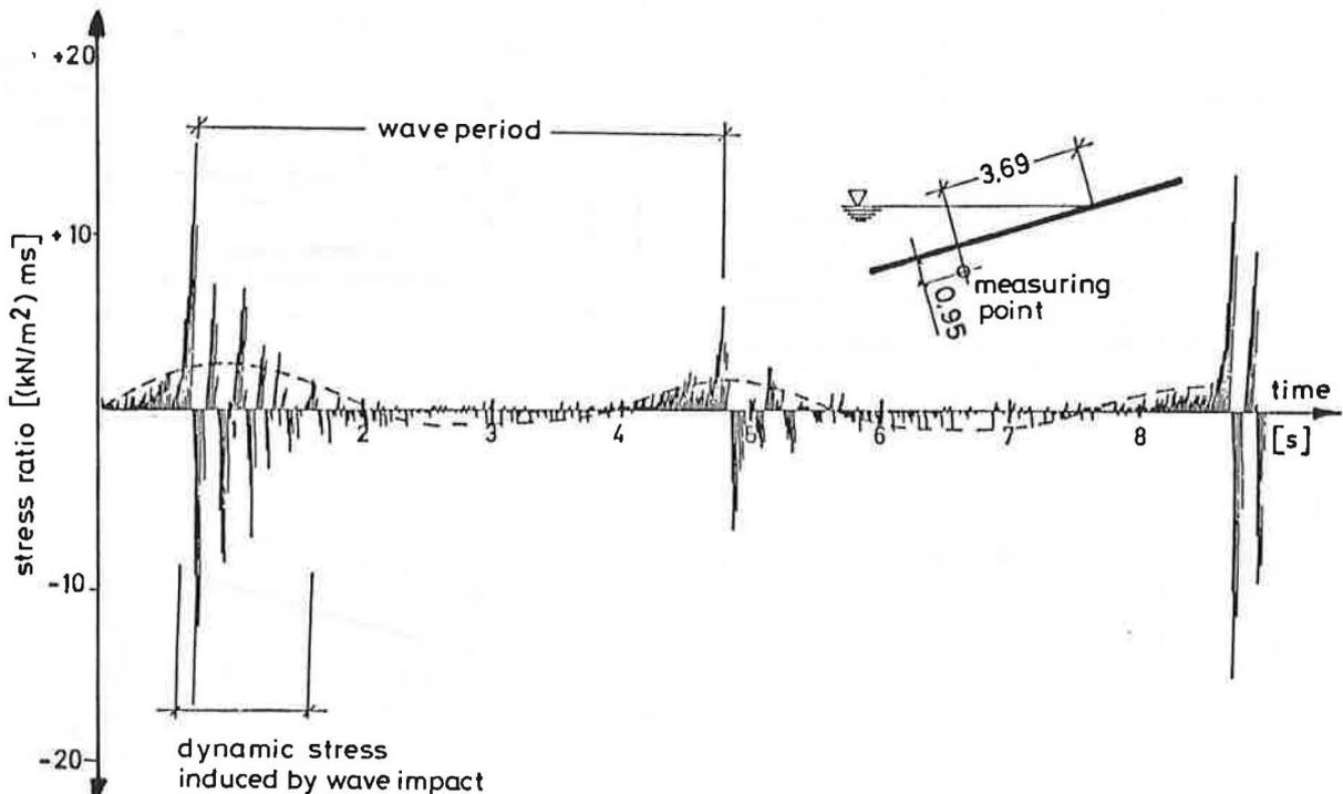
Fig.6: stress ratio of change of stress in Fig.4, level B, profile 3 (see Fig.2) dueto wave H=1.25 m and T=4 s
