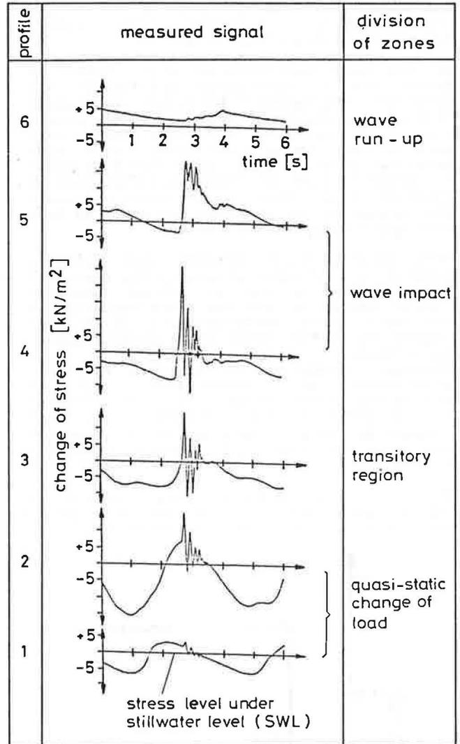
Fig.5: change of stresses in level A, profiles 1 to 6,  $H=1.75$  m and  $T=6$  s
