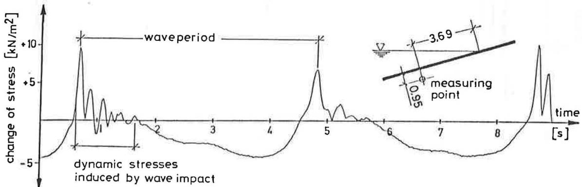
Fig.4: change of stress in level B, profile 3 (see Fig.2) due to wave  $H=1.25$  m and  $T=4$  s
