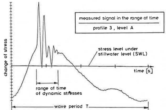
Fig.7: characteristic stress sequence near to the breaking point
