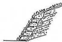
Fig. 16 Screen walls in front of rock faces
