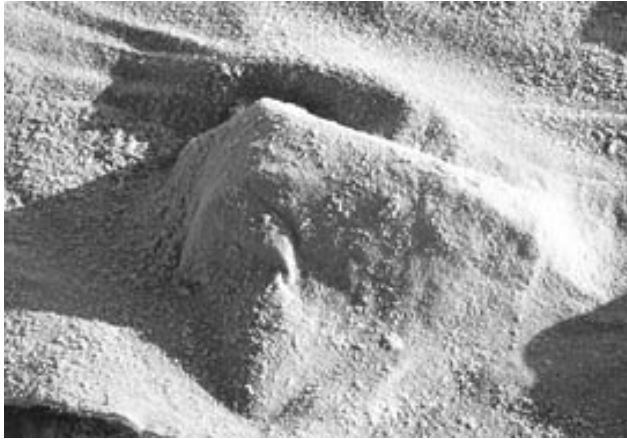
Figure 4. Lacanau : reverse imprint of a rock placed on the geotextile.
