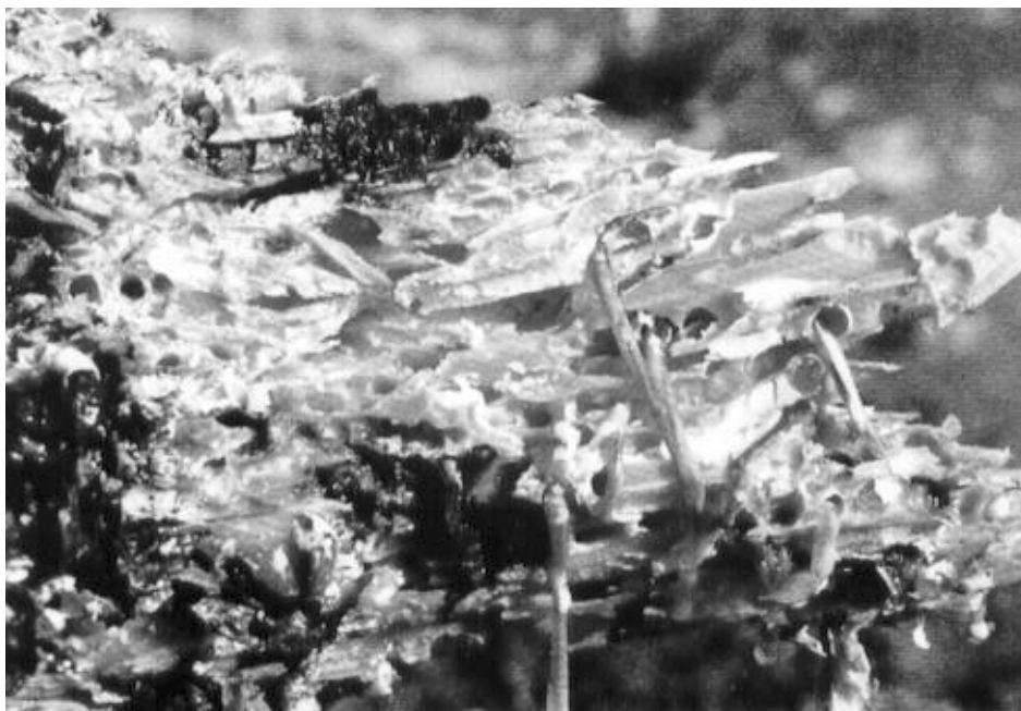
Figure 4: Pine wood completely destroyed by Teredo (Sordyl et al. 1998)
