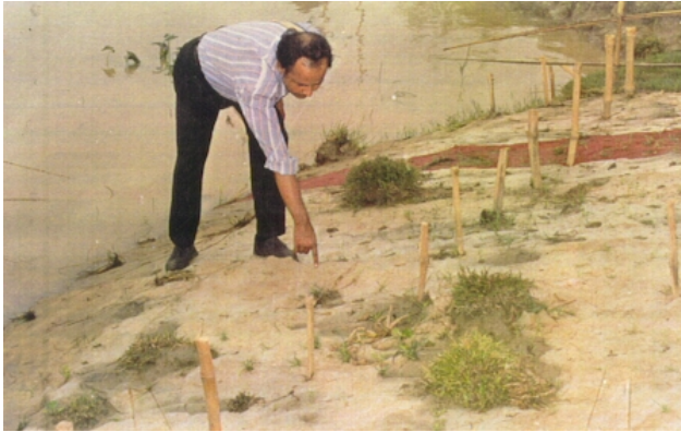
Photo 1. Observing growth of grass through the fabric 15 days later after layout (sabujdeep Project)
