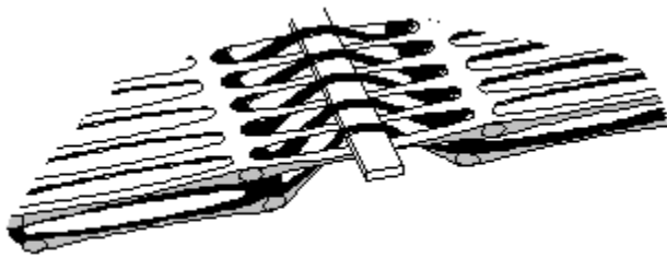
Figure 3: Connection between two geogrids using a bodkin connection
