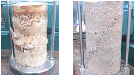
Figure 4. Different failure modes for 7% cement-stabilized fiber-treated (left) and fiber-untreated (right) soils
