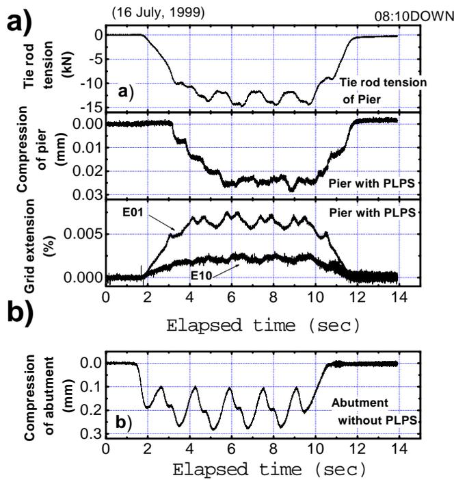
Fig. 4 Behaviours of a) the pier and b) the abutment during a train passing after 2years of service (July, 1999)
