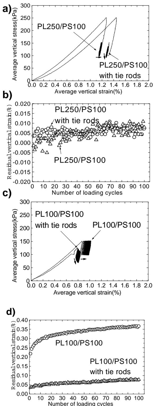
Fig. 8. Test results with and without tie rods
