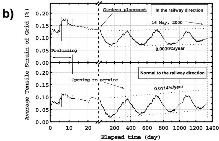
Fig.3 Long-term behaviours of a) the pier and abutment and b) average of grid tensile strain of the pier in each horizontal
