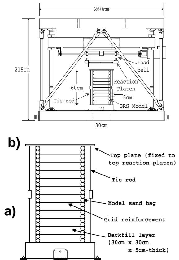
Fig. 5. a) Loading frame and b) GRS pier model.
