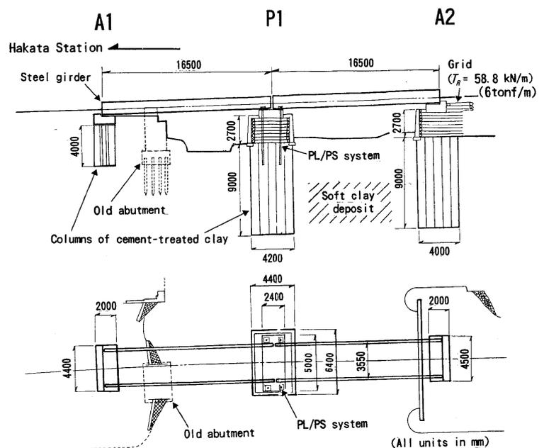
Fig. 1 Maidashi bridge with PLPS reinforced soil pier.
