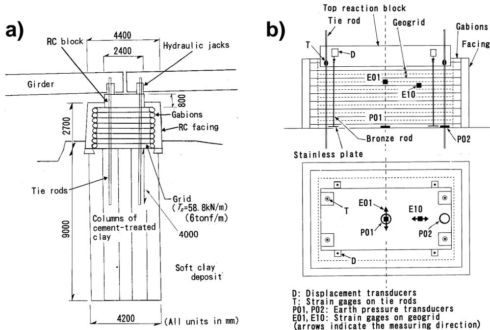
Fig. 2 a) Details of the pier, and b) arrangement of the instrumentation described in this paper.
