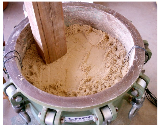
Figure 3 – Soil compaction inside the calibration chamber.
