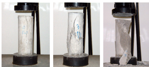
Figure 5. Fractured feature of FRC with reinforcement fibers.
